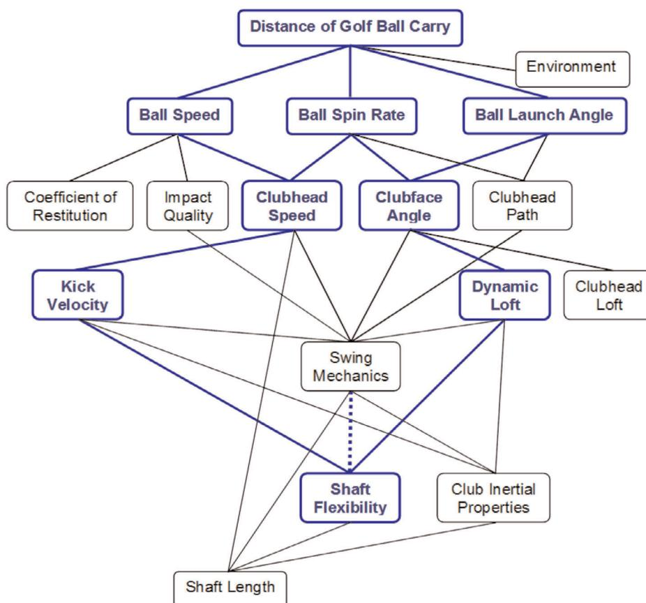
Figure 1. Flow Diagram Illustrating How Shaft Flexibility Influences the Distance a Golf Ball will Travel in the Air Following Impact with a Driver. Lower factors affect the higher factors of which they are connected. Environment refers to factors such as air temperature and wind. Impact quality refers to the location of impact on the clubface. Shaft flexibility may affect the feel of the club during the swing which could alter the golfer's swing mechanics.
